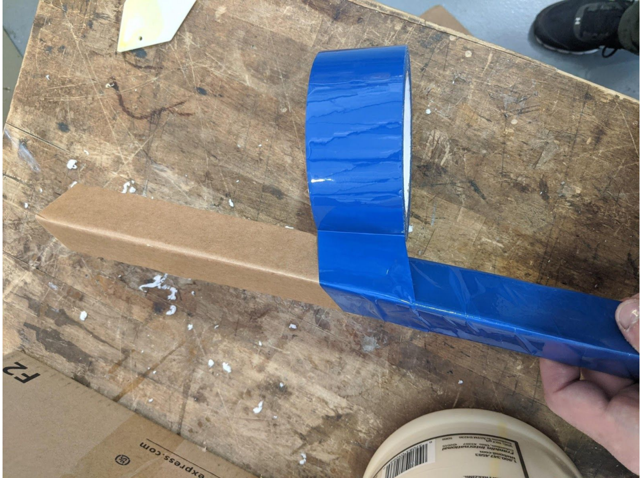
Figure 6 - Folding and Taping Fuselage
