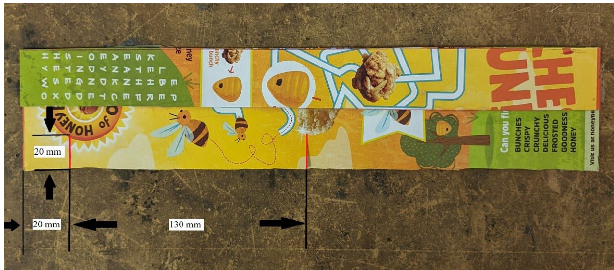
Figure 2 - Control Surface Cut Dimensions (Wing)
