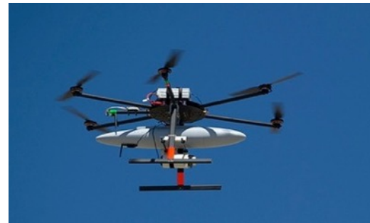
Mid-efficiency hover: Large hexacopter built by VT
