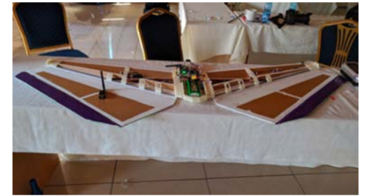
The EcoSoar aircraft skin is comprised of a foam core material and paper/plastic skin
