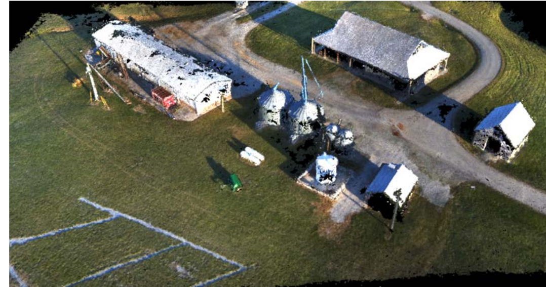
This scene has missing points due to poor texture in the roof of the building on the left
