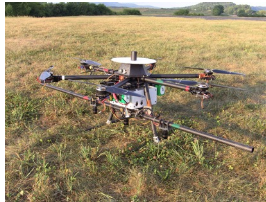
The same aircraft carries a radiation detector (left) and a SBC + stereovision system (right)
