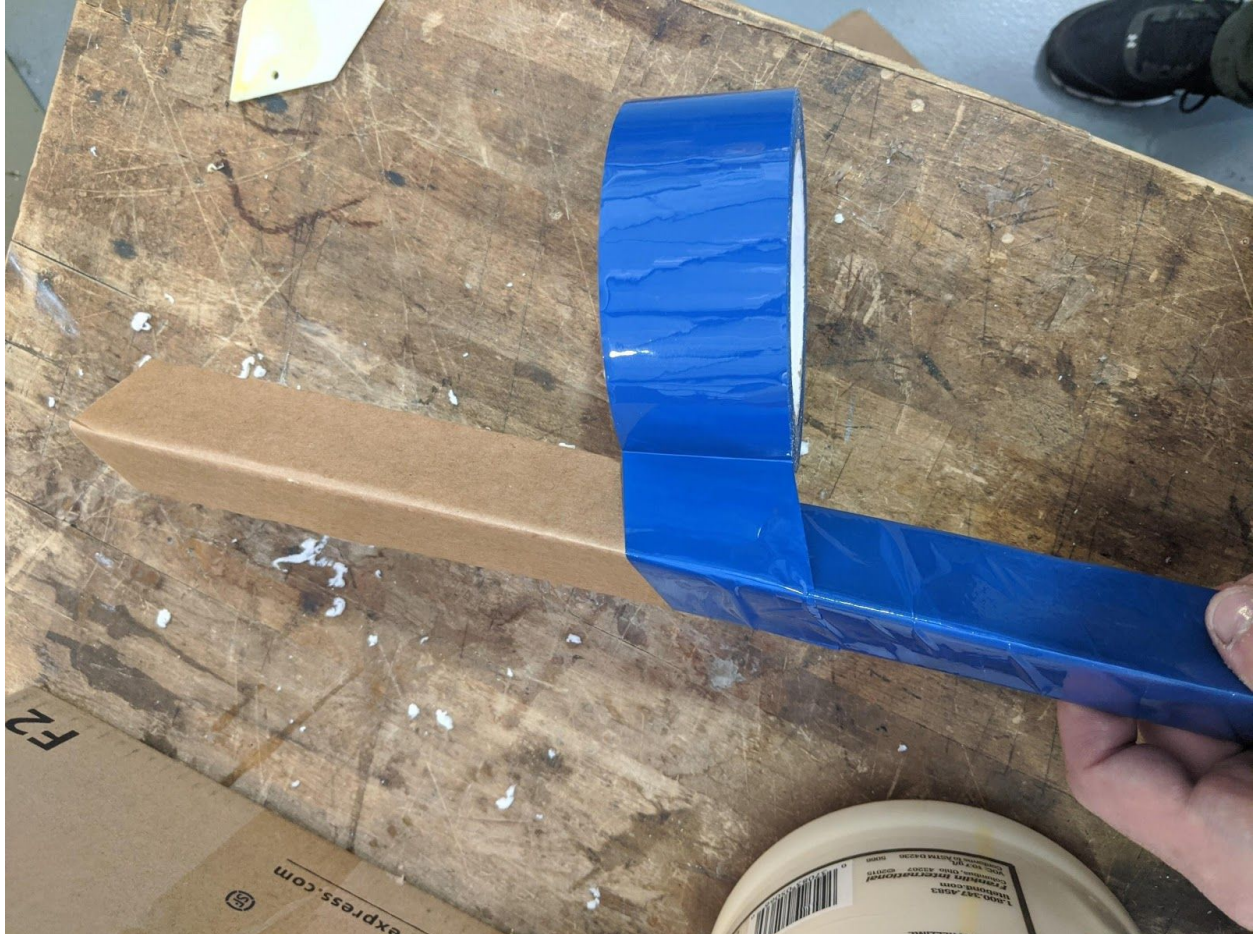
Figure 6 - Folding and Taping Fuselage
