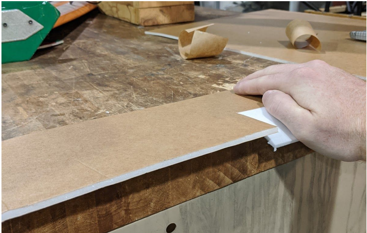
Figure 1 - A posterboard control surface molded to better fit in the wing
