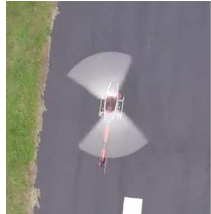
The rotor of the Yamaha RMAX is not symmetrical in this image due to the rolling shutter
