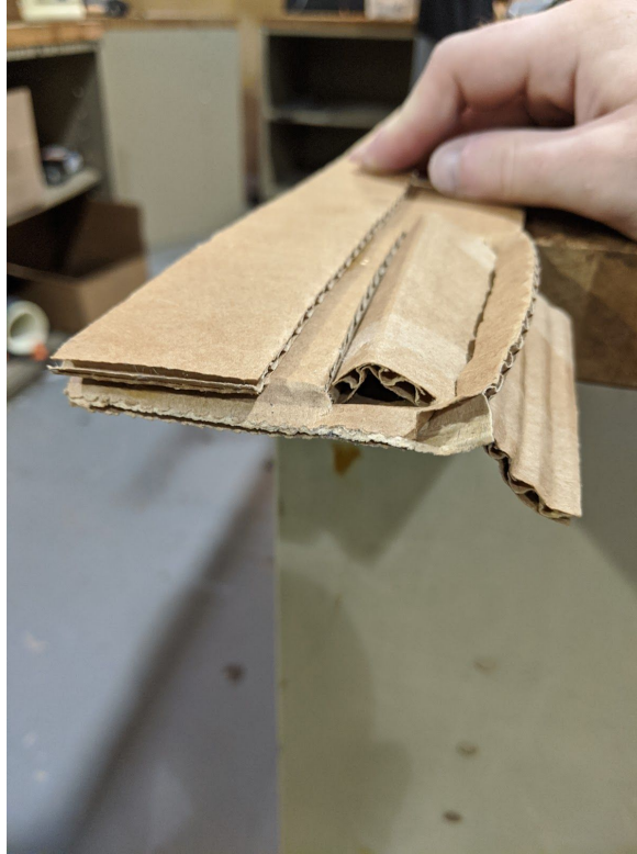
Figure 4 - Wing with aileron slotted through
